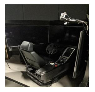
*The RDS* – 1000 *driving simulator* (*Real-time Technologies, Inc.*) *driving simulator*.
