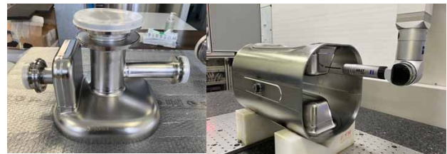
Figure 5: Subcomponents of Pre-Series cavities during manufacturing and inspections.
