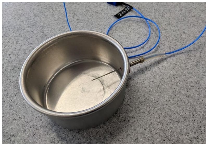
Figure 3-7 Modified cake tin with a needle probe to allow internal temperature measurement of the cakes while baking.
