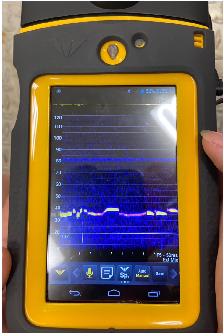
Figure 3.5 Screen of the Walkabout showing a spectrum from a tickling session. Image taken by Gabrielle Johnston
