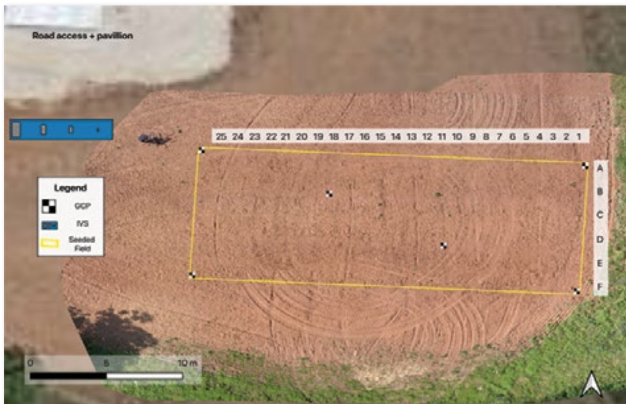
FIGURE 4. Permanent seeded field map displayed as an orthomosaic on a satellite map. The blue square shows the location of the IVS relative to the field. There is a pavillion for field operation logistics and gravel road access to the site.
