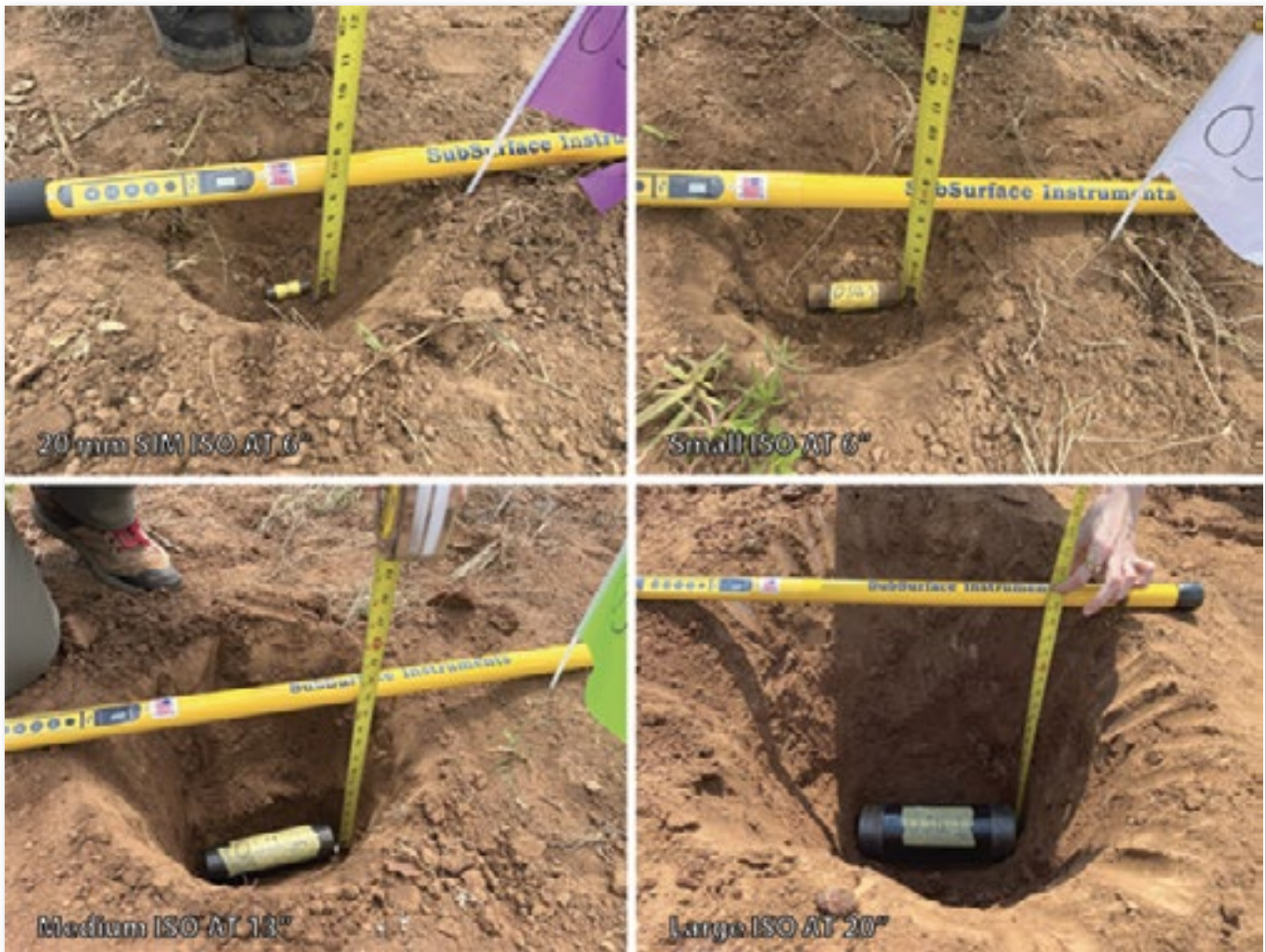
FIGURE 5. Instrument verification strip, ISO buried at recorded depths of 6 inches (15.2 cm), 13 inches (33.0 cm), and 20 inches (50.8 cm) respectively.
