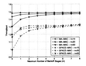
Figure 3.12: Throughput vs Backoff Stages
