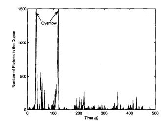
Figure 2.7: Access Point Queue Evolution for Access Point Serving 4 Stations
