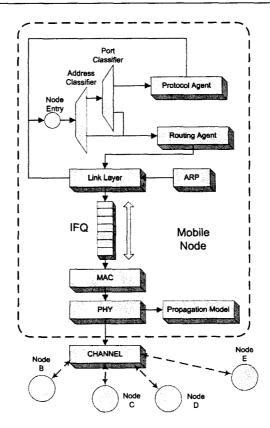
Figure 2.8: Mobile Node Model in ns-2
