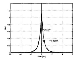
Figure 4.10: Voice Downlink Jitter for Station 4
