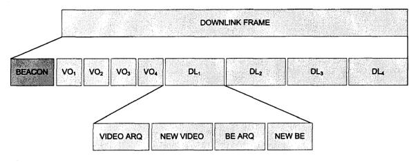
Figure 4.3: TV-TDMA Downlink Frame
