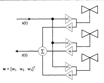
Figure 2.3: Radio Structure for Specified MIMO System
