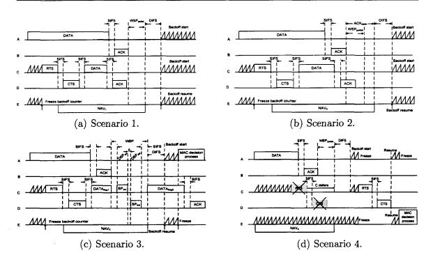
Figure 3.5: Timing diagram of MAC decision process for secondary stations.
