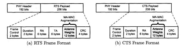
Figure 3.3: Access Control Packets
