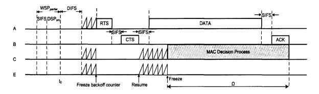
Figure 3.4: MA-MAC scheme timing diagram.
