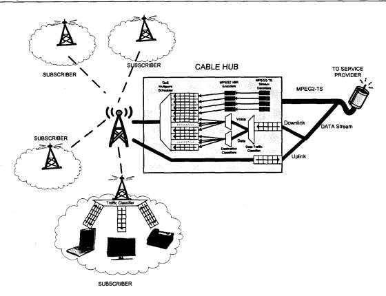
Figure 2.4: Proposed Point-to-Multipoint Wireless Video System
