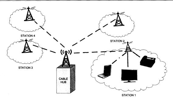
Figure 4.1: Point-To-Multipoint Wireless Network Scenario
