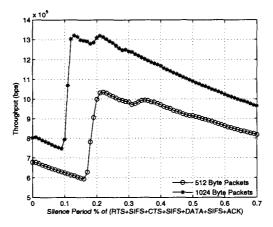
Figure 3.1: Throughput vs. Silence Period - 20 Stations - 1Mbps
