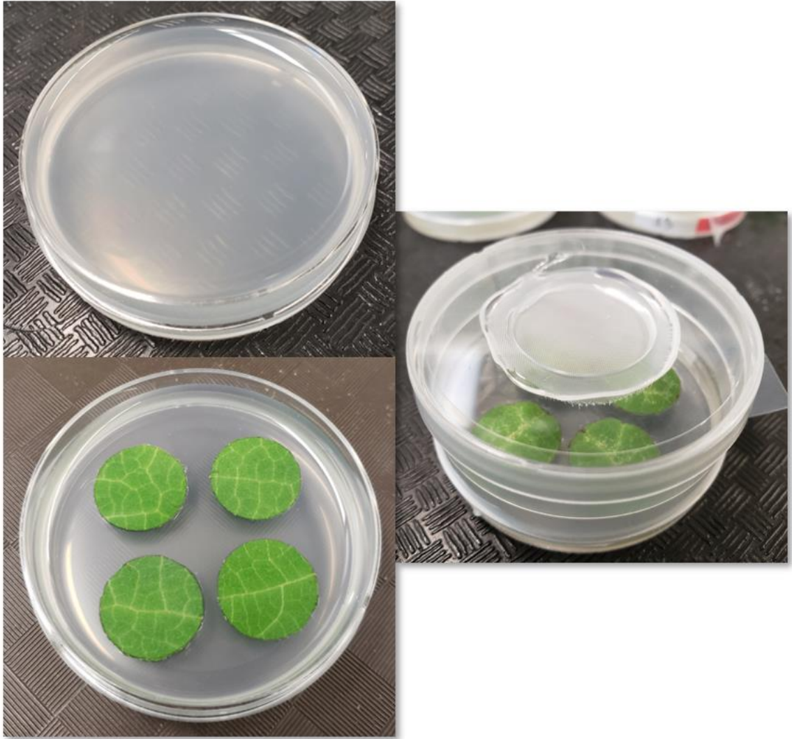
Figure 2.4: Ovicidal experimental setup. 60 × 15 mm Easy Grip Tissue Culture Dish with 0.8 % agar to support 1.5 cm diameter leaf disks. Capable of supporting leaf disks for approximately 12 days.
