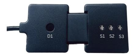
Figure 6: Close-up of source-detector parings on the Portalite fNIRS system. D1: Detector 1, S1: Source 1 (30mm), S2: Source 2 (35mm), S3: Source 3 (40mm).
