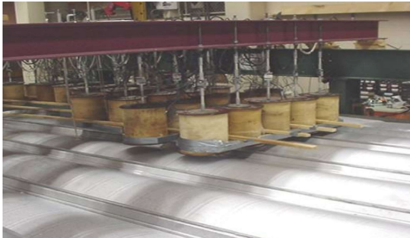
Figure 24: Electromagnetic uplift testing configuration on standing seam metal roof (Sinno, 2008).
