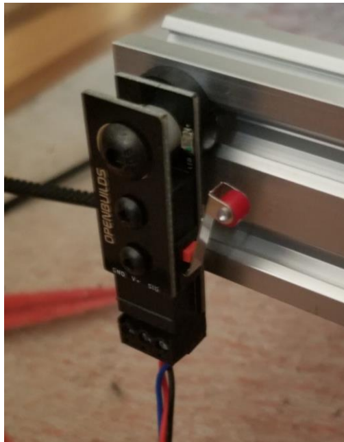
Figure 36-Limit switch positioning on a V-slot
