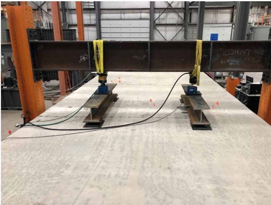
Figure 7.15: Photograph of the symmetric flexural test
