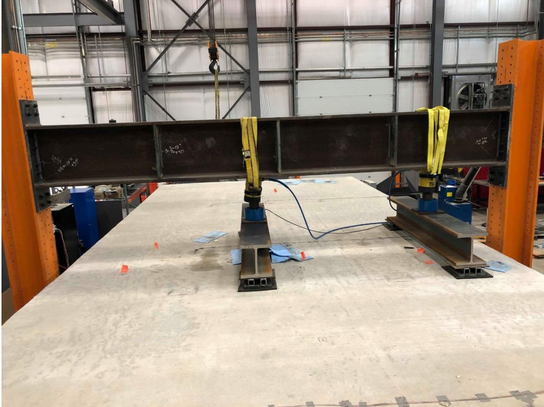
Figure 7.20: Photograph of the eccentric flexural test
