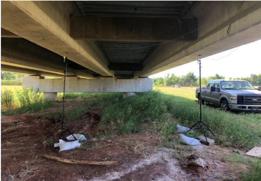
Figure 6.5: Testing setup for SH 4 load test.
