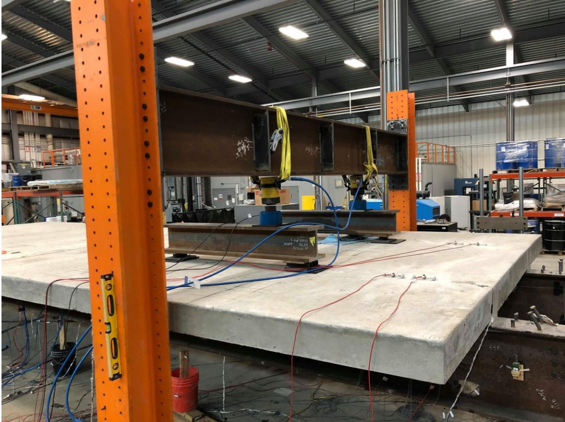
Figure 7.23: Photograph of the symmetric shear test
