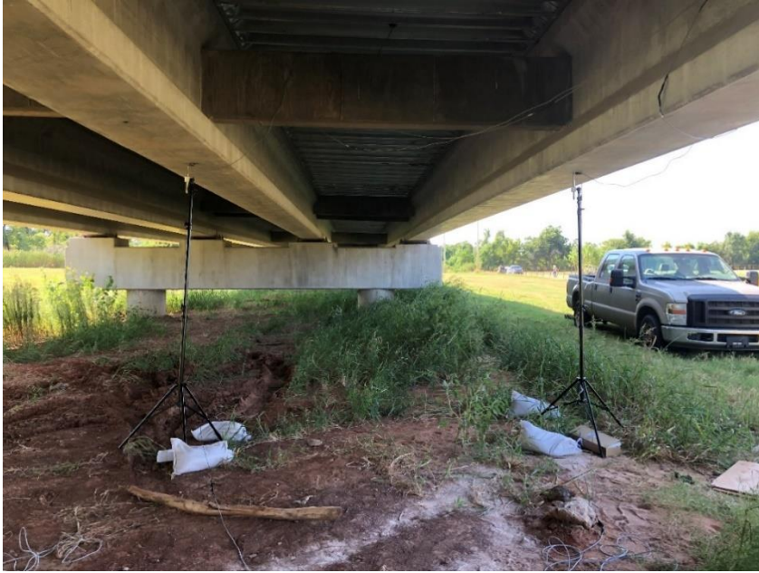
Figure 3.21: Testing setup for SH 4 load test.
