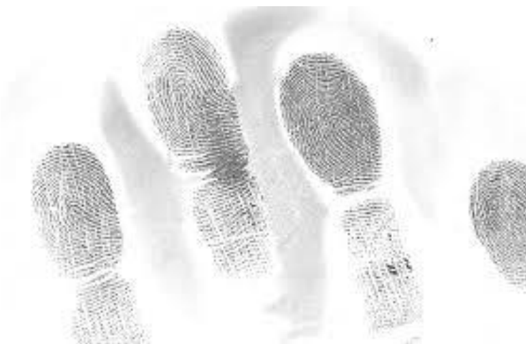
Figure 7 Halos of powder around fingerprint, (Watson, 2008).
