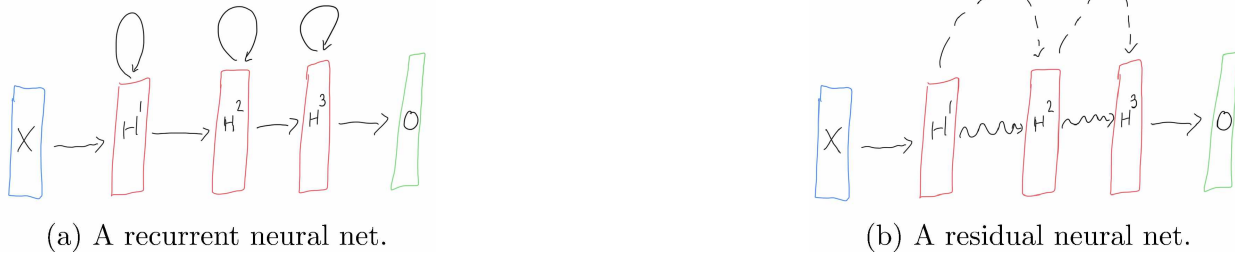
Figure 2.4: (a) The composition diagram of a recurrent neural net with 3 recurrent hidden layers, where recurrent connections are denoted by loops, and (b) the composition diagram of a residual neural net with 3 hidden layers, where skip-connections are denoted by dashed lines and residual connections are denoted by squiggly lines. In both figures, blue denotes the input layer, red denotes hidden layers, and green denotes the output layer; nodes within layers are excluded for simplicity.
