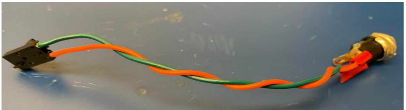
Figure 3.13: Finished Power Cable (Image Courtesy of Dogacan Ozturk)
