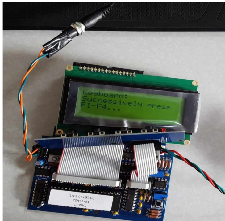
Figure 3.10: SAM-III ready for software setup. The steps will need to be followed on the LCD.
