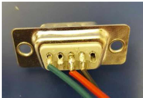
Figure 3.22: Soldered wires on Plug (Image Courtesy of Austin Cohen)
