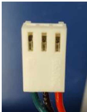
Figure 3.23: Wires in Housing (Image Courtesy of Austin Cohen)
