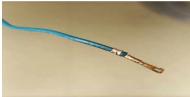
Figure 3.9: Terminal Contact Around Wire (Image Courtesy of Austin Cohen)
