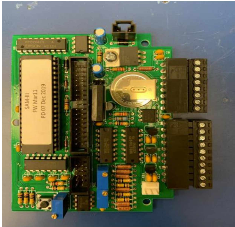
Figure 3.8: Finished main PCB. Some of the older boards are green, while the newer boards are blue.
