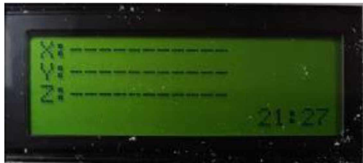
Figure 3.11: Final screen. None of the sensors are installed at this point in the construction process, so the readings should be empty at this moment.
