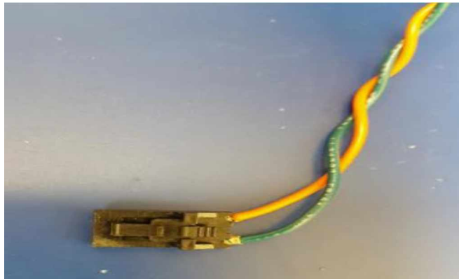
Figure 3.10: Terminal Contacted Wires into Housing (Image Courtesy of Austin Cohen)
