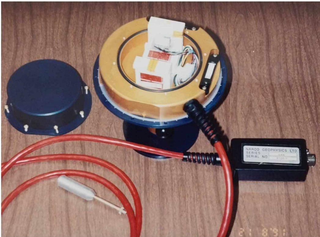
Figure 3.2: Narod photo. The lid has been removed to show the internal components of the device. Adapted from Osborn (1991).
