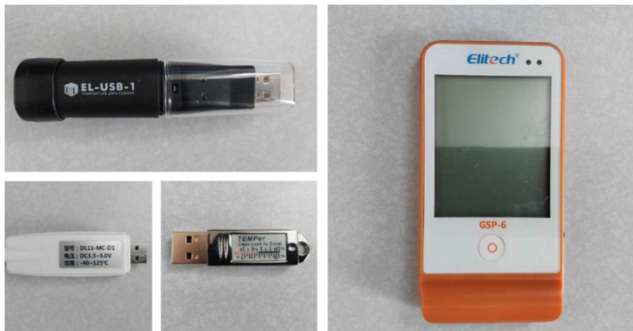
Figure 4.5: Options tested for temperature data collection. [Top left] Lascar EL-USB-1. [Bottom left] Taidacent MODBUS. [Bottom Middle] TEMPer Gold. [Right] Elitech GSP-6.
