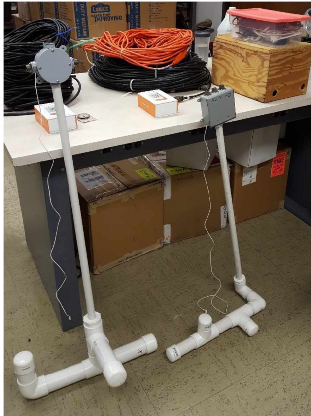
Figure 5.2: A-Type (Left) and L-Type (Right). All the cabling required for operation is shown in the background.
