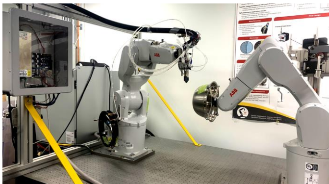
Figure 1. Machinery and system setup for non-planar printing of continuous fibre using 6-axis robotic arm.
