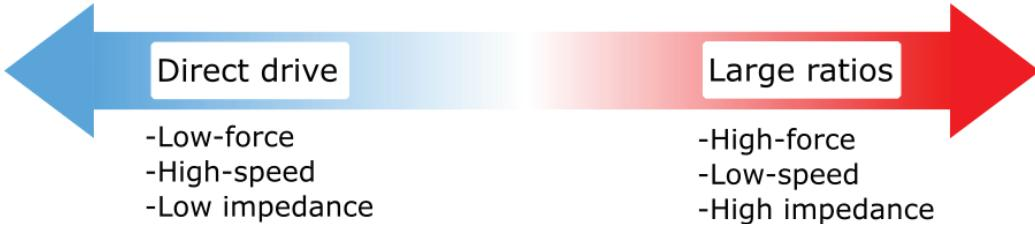
FIGURE 3.1 Trade-offs of geared motors with a fixed reduction ratio.
