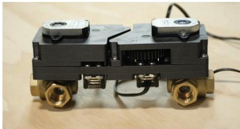
(a) Two three-way ball valves actuated with servo motors;
