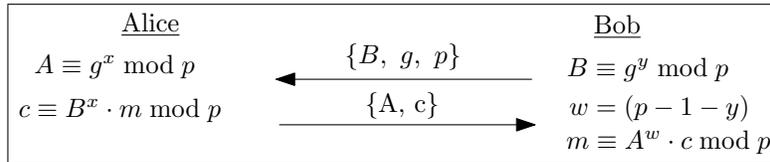
Figure 1. The ElGamal Encryption and Decryption Protocol.
