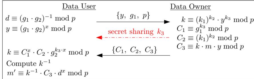
Figure 2. The Flow of Enhanced ElGamal Scheme.
