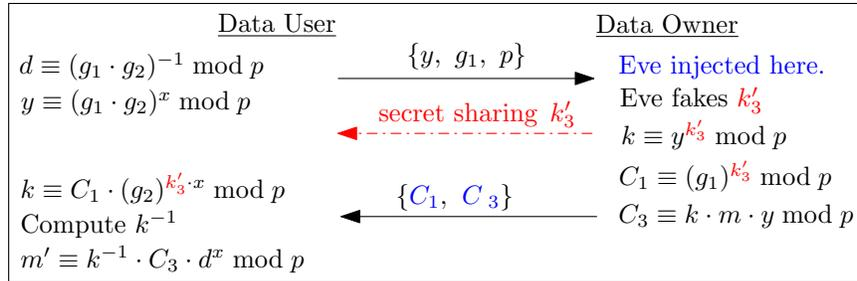
Figure 4. The insider attacks Enhanced ElGamal Scheme.
