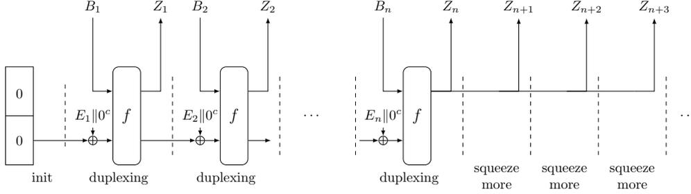
**Figure 2:** Illustration of the OD construction. Note that neither the padding of the input blocks  $B_i$  nor the encoding of the trailer  $E_i$  is explicitly depicted in this figure, please see Algorithm 2 for more details on this.
