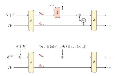
Fig. 33: Illustration of a proof step for  $SCHWAEMM_{IV}$  (Theorem 11). SCHWAEMM<sub>IV</sub> is represented as a plain sponge as is shown for the first XOR in the above figure.
