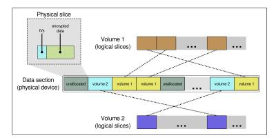
Fig. 4: Shufflecake's data section layout and slicing.
