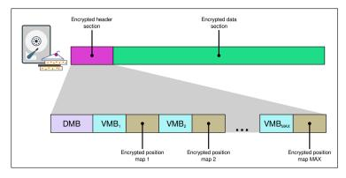
Fig. 3: Shufflecake's disk layout overview.
