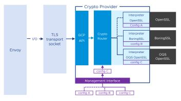
Figure 6: Cryptographic Provider Integration into Envoy
