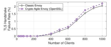
Figure 8: TLS handshake failure rate vs Number of consecutive clients
