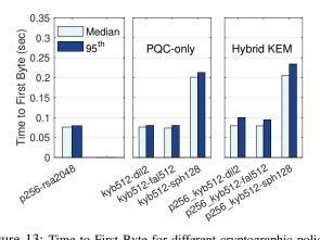
Figure 13: Time to First Byte for different cryptographic policies
