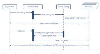
Figure 5: Sequence diagram of the CP component prototype consumption in a Server establishment use-case.
