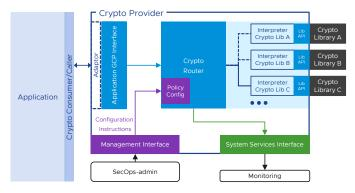
Figure 2: Generic Cryptographic Provider Functional Diagram
