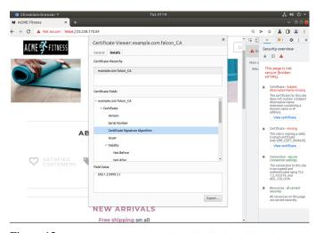
Figure 12: ACME app page authenticated with the PQC Falcon-512 digital signature algorithm
