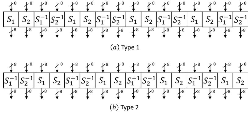
Fig. 1: Two types of S-box layers in ARIA
