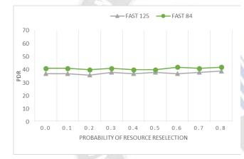
Figure 6. Effect of changing probability of resource reselection parameter on PDR
