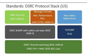
Figure 1. DSRC Protocol Stack
