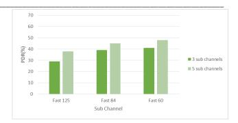
Figure 7. Effect of changing the number of sub-channels on PDR
