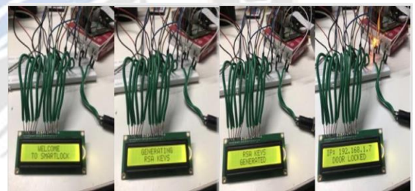
Fig. 3 Hardware Setup for System Initialization
