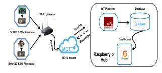
Figure 6. Architecture of deployed IAQ monitoring system
