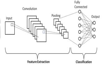
Figure 2: Typical CNN architecture
