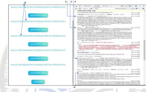
1: List of Sender's Blockchain wallet addresses 2: Private key of Receiver 3: Public key of Receiver for symmetric key encryption 4: Decryption Process 5: Decryption key for original data file conversion. Figure 2: Using the private key with a symmetric key to decrypt data
