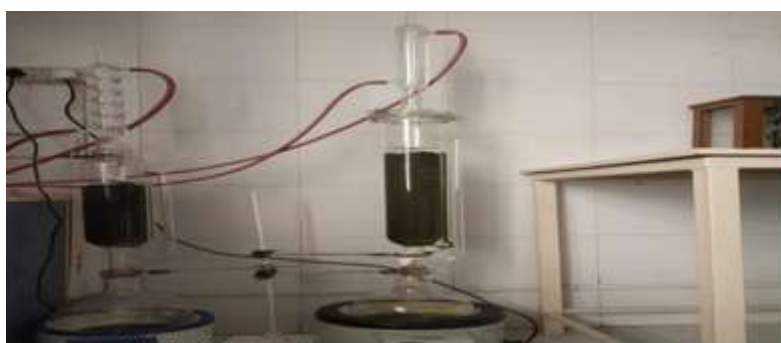
Figure 01: Soxhlet extract apparatus assembly for extraction of phytochemicals from Plant Root Extract
