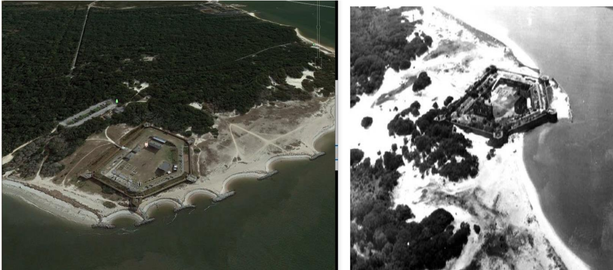
Figure 17: Comparison of shoreline around Fort Clinch in 2021 (left) and 1940 (right). (Google Earth/State Archives of Florida)
