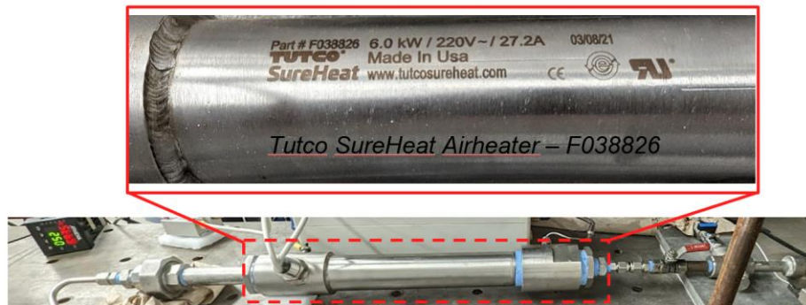
Figure 10 : Picture of Air heater with Thermocouple, DAQ system
