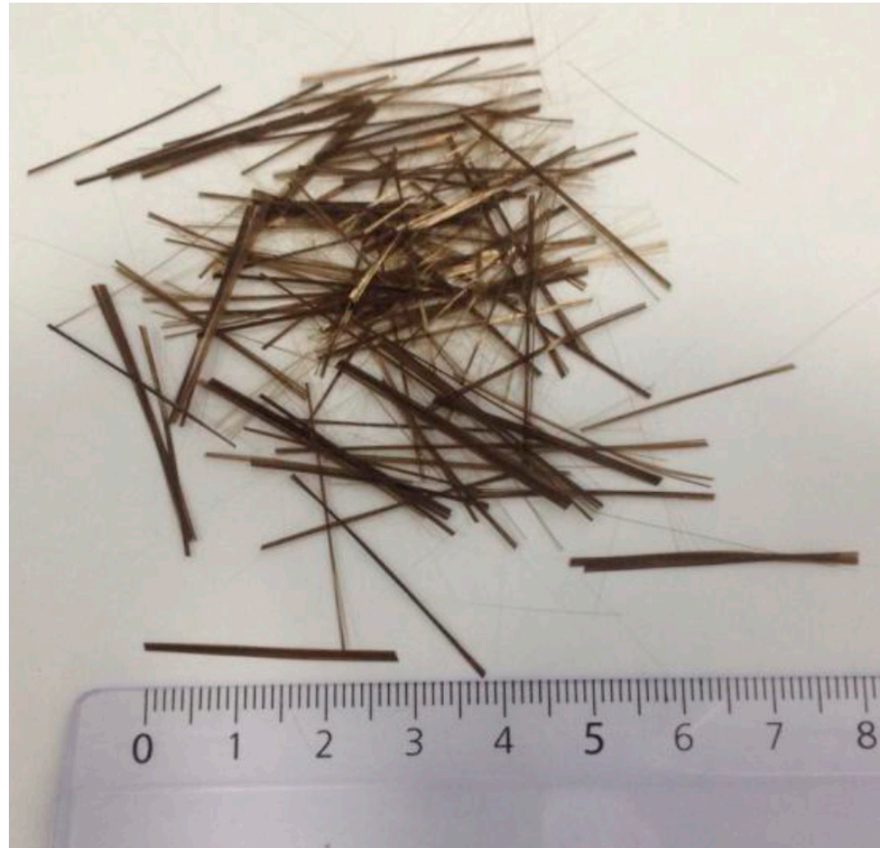
Figure 1. Sample of recycled slate fibers used to make the composites used in this study. The fibers are about 30 mm long and have an average diameter of 15 to 23 \mu\text{m} .
