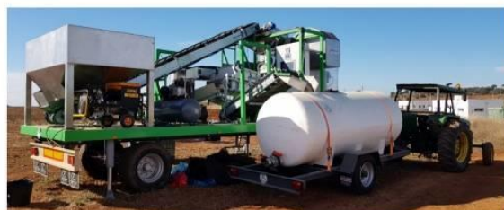
Fig. 7. TRCS and TST trailers located in a plot to test the performance during harvesting season.
