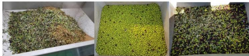
Fig. 14. Fruit entry in the hopper (left) and 'A' quality output (centre) and 'B' quality output (right).
