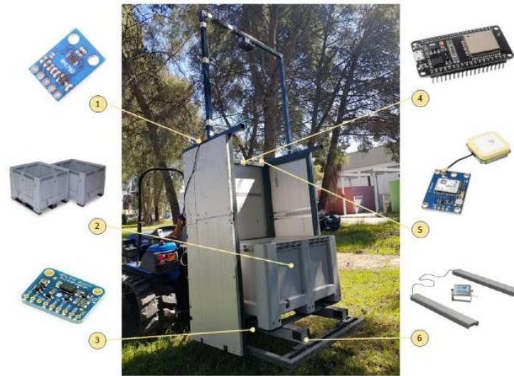
Fig. 1. Structure of the commercial system mounted on the tractor for installation of the measuring systems and auxiliary elements. 1.-Luxmeter, 2.-Big box, 3.- Accelerometer, 4.-Microcontroller, 5.-GPS, 6.- Load cell.
