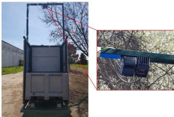
Fig. 2. Yield monitor prototype developed with the commercial system over a metallic structure and a big box for the stored fruit (left). Detail of the 3D camera (right).
