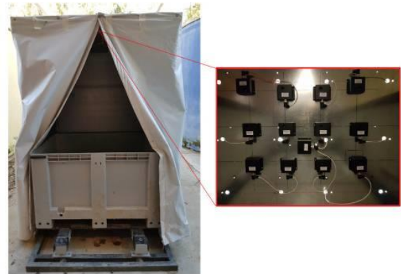
Fig. 3. Yield monitor prototype developed with the experimental system over a metallic structure and a big box for the stored fruit (left). Detail of the ToF sensor array (right).
