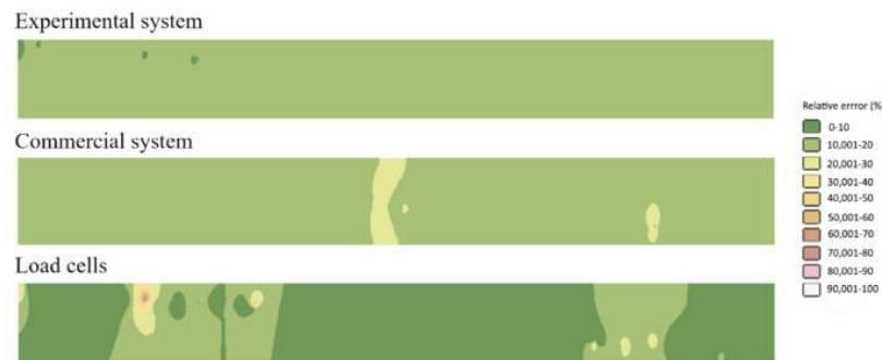
Fig. 15. Variation in weight relative error considering the load transported during the dynamic test for different systems.
