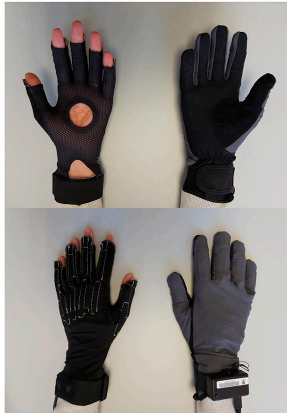
Figure 2. Same participant wearing a CyberGlove (left hand) and a VMG30 (right hand).
