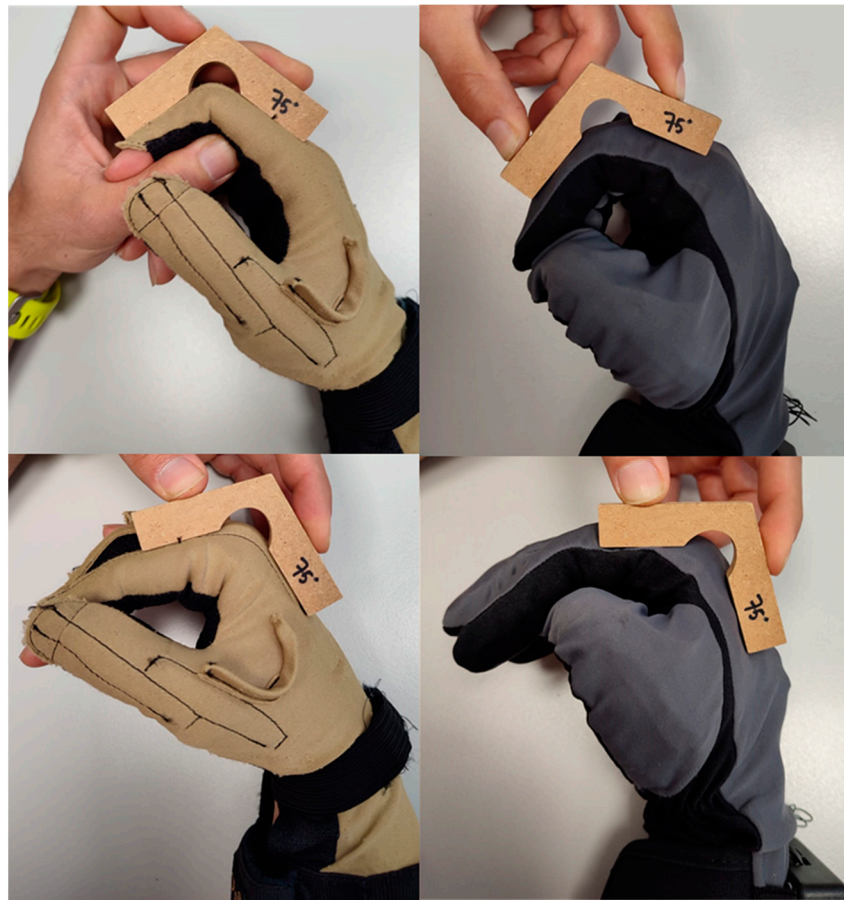
Figure 6. One of the accessories for data glove calibration, according to a previously validated protocol [1]. The same accessory calibrating index MCP flexion and PIP flexion for CyberGlove (left) and VMG30 (right).
