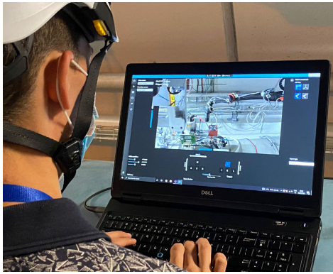
FIGURE 5. The operator using the 2D interface and controlling a remote manipulator in the LHC. The cameras' view, control modes selection, keyboard input mapping, speed setting, and numeric joint positions can be seen on the laptop screen.
