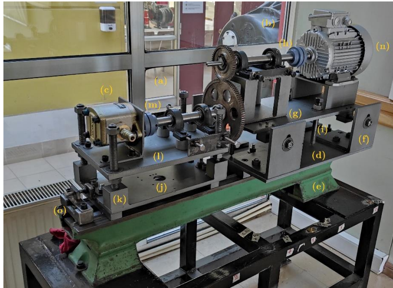
Figure 7. Testing workbench for misalignments. (a) Reactive side (b) Motor side (c) Gear pump (d) Lower base plate (motor) (e) Machine bed (f) L plates (g) Upper base plate (motor) (h) Flexible coupling (motor) (i) Vertical screws (motor) (j) Base plate (reactive side) (k) Support hubs (l) Top plate (reactive side) (m) System for axial movement of the reactive side. (n) Motor power.
