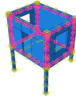
Fig. 6 - Applying tie constraints for all surface that were in contact
