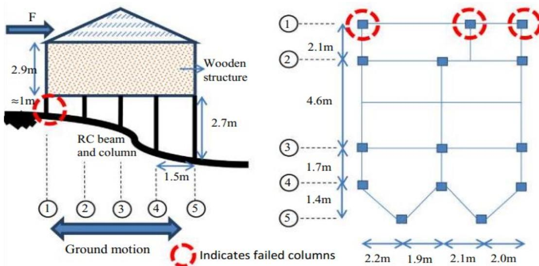
**Fig. 3 - Building configuration measured onsite and columns grid as reference (a) side elevation, and; (b) building plan [1]**
