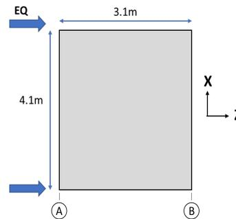
Fig. 10 - Plan view of stilt house model
