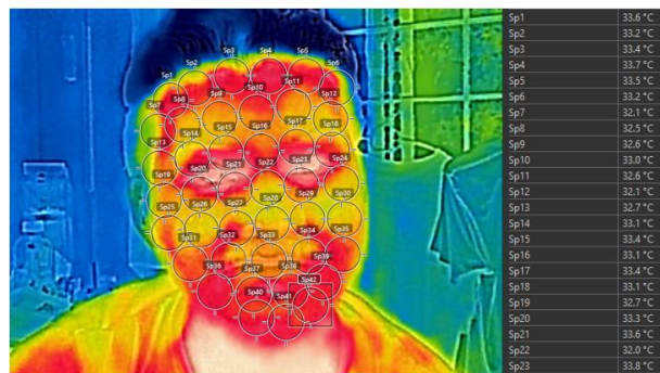
Fig. 10 - Region of interest with spot measurement
