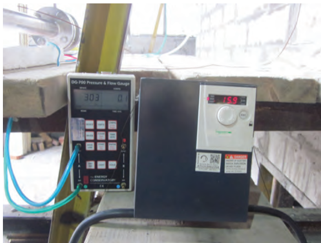
Figure 8: Frequency regulator and device for measuring the pressure difference
