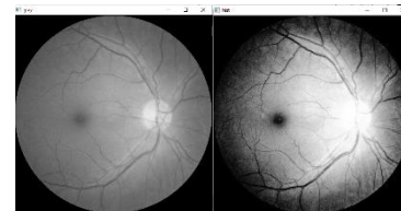
Figure5 shows the result of histogram equalization of the gray image
