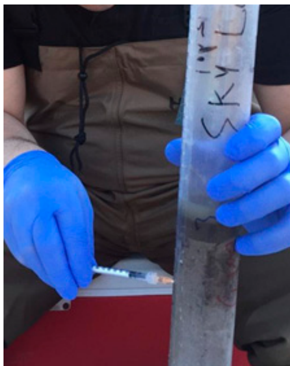
Figure 4. Injecting Hg tracer isotopes into a sediment core.
