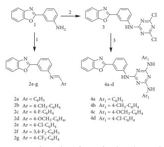
SCHEME 1: Synthetic pathway of **2a–g** and **4a–d**. Conditions and reagents: (1) ArCHO,  $CH_3CH_2$  OH,  $CH_3COOH$ , reflux, 4 h; (2) cyanuric chloride, acetone, rt, 1 h; and (3) aryl amine,  $K_2CO_3$ , dioxane, reflux, 12 h.
