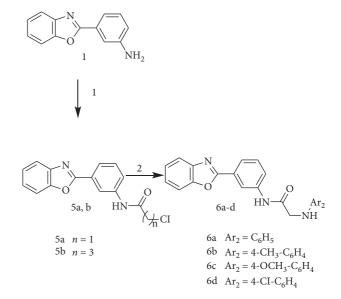
SCHEME 2: Synthetic pathway of **5a-b** and **6a-d**. Condition and reagents: (1) acid chloride,  $K_2CO_3$ , dimethyl formamide, rt, 24 h; (2) aryl amines, TEA,  $CH_3CH_2$  OH, reflux, 12 h.
