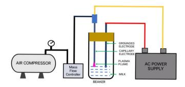
Figure 1. The schematic of microplasma discharge setup
