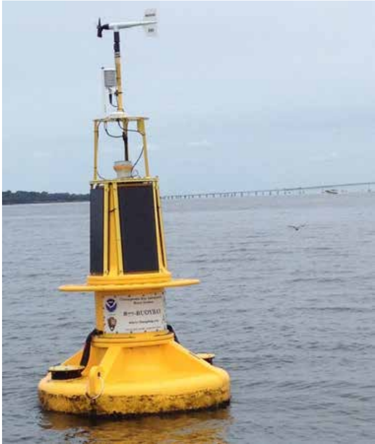
Figure 2: Annapolis CBIBS buoy deployed near the mouth of the Severn River. (Photo courtesy of C. Reid Nichols)
