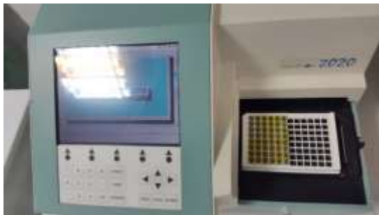
Figure1: Added stop solution to each well. The color in the well changed from blue to yellow.
