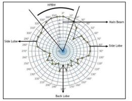
Figure 25. Radiation Pattern of 2x4 Element Rectangular H-Slot Array Microstrip Antenna
