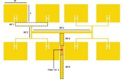
Figure 5. Antenna microstrip rectangular H-Slot array
