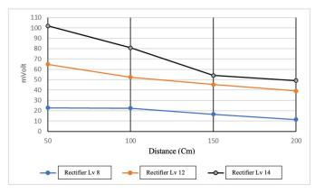
Figure 28. Graph of rectenna average voltage output test results
