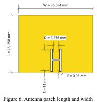
Figure 0. Antenna paten length and width
