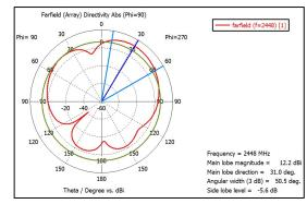
Figure 20. Radiation pattern simulation results
