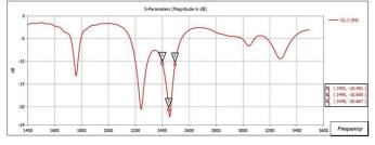
Figure 16. Return loss simulation results
