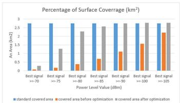
Figure 7. Graph of Surface LTE Network Coverage Percentage Before and After Optimization
