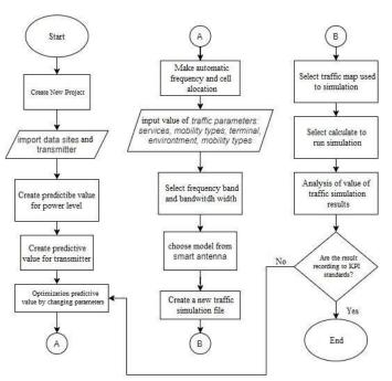
Figure 2. Modeling Flowchart and Traffic Simulation Modeling
