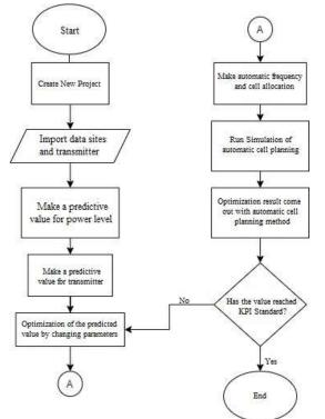
Figure 1. Coverage Modelling Diagram with Automatic Cell Planning Method
