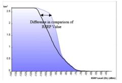
Figure 12. Histogram Graph of Comparison of RSRP Values Before and After Optimization
