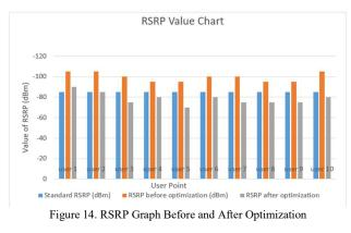
Fig. 14 is a graph of the RSRP value optimized by the Automatic Cell Planning method. The 10 users who are actively connected to perform network service activities, the results reach an average value of -100.5 dBm while the standard KPI value for the RSRP value is -85 dBm. This means that the RSRP value in optimization with the Automatic Cell Planning method is better than the average value obtained from the drive test after optimization by adding sites and changing azimuth.
