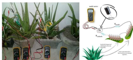
Figure 2. Experimental setups (from left to right: Nitrogen-based, Potassium-based, Phosphorus-based, No fertilizer)
