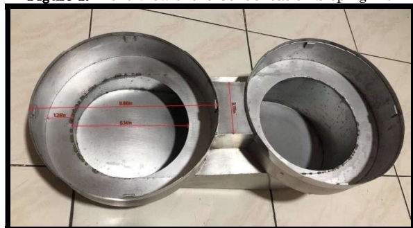
Figure 2. Bottom View of the Condensation Sloping Lid
