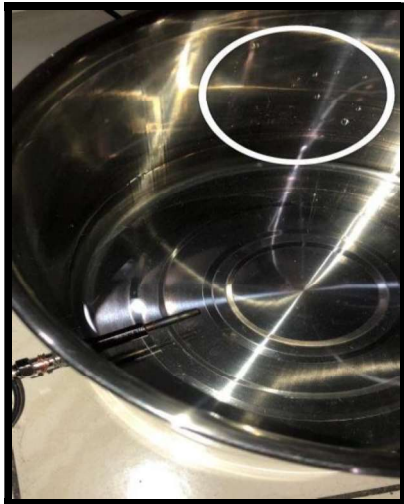
Figure 9. Condensed Water Droplets on the Unsubmerged Wall of the Container
