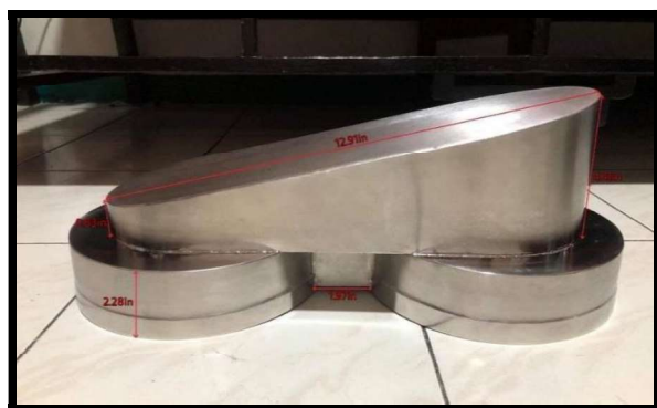
Figure 1. Front View of the Condensation Sloping Lid
