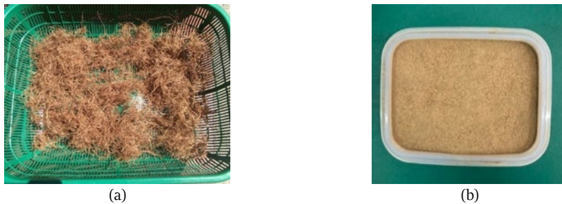
Figure 1. (a) The untreated OPEFB before, and (b) after grinding and sizing
