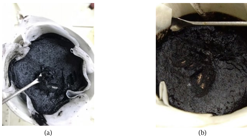
Figure 2. (a) Hydrolyzed OPEFB (b) delignified OPEFB
