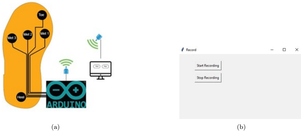
Figure 2: (a) Schematic diagram of the proposed system. (b) GUI designed for the system.
